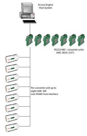
For applications where multiple AMCs are required, up to eight (8) AMC can be connected via RS485 (2 or 4 wire) using the RS232 to RS485 interface converter.
